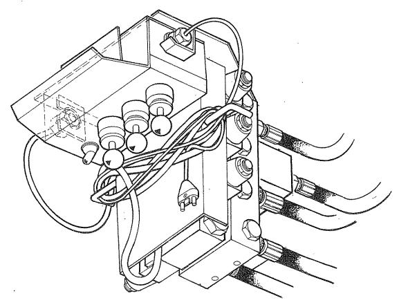
Disconnect electrical plug within cab and unhook the control box from its mounting. Coil the cables around the storage spigots on the armhead valve and turn the box upside down and lift into place in the cradle brackets beneath the protective shroud.
