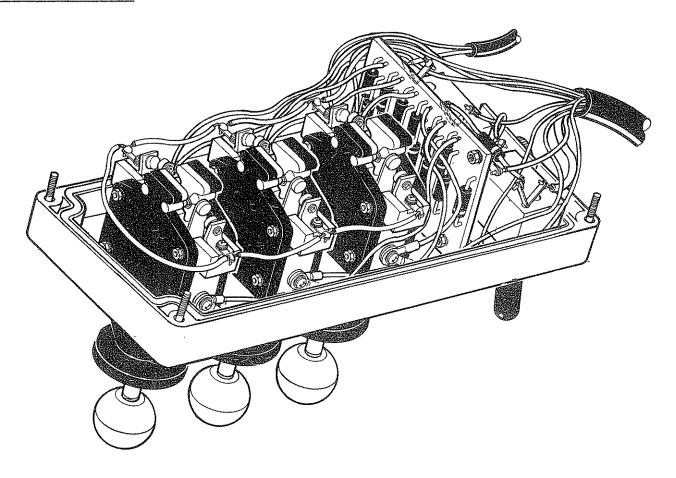
The control unit contains three lever switch units each comprising two contact breaker assemblies. Little maintenance should be required other than light cleaning of the contact points with a suitable points cleaning file if switching should become intermittent after a prolonged period of use.
