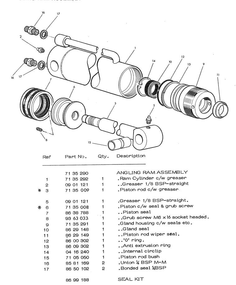
\* When replacing a piston rod or a piston on machines prior to serial No 04 GG 77 a complete piston/piston rod assembly is necessary Part No. 71 35 106.
