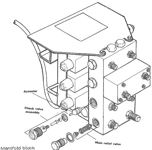
This contains the main relief valve and pilot operated ball check valves. The main relief valve is pre-calibrated to 1800 psi (125 Bar) and is non-adjustable.
