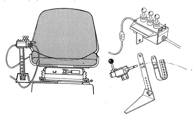
The supply cable with the disconnect plug should be connected to the tractor's electrical system prefereably at the fuse box or the ignition switch where it can be switched off with the tractor's isolation key.
