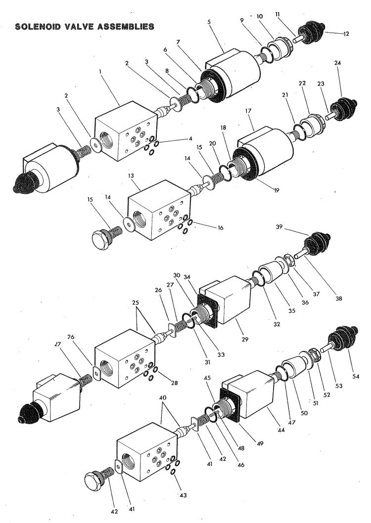
Two different types of solenoid assemblies are fitted depending on supply availablility. Both assemblies are directly interchangeable on the manifold block and have the same assembly part number. Individual spares for a particular solenoid are not interchangeable and care should be taken in identifying the correct one.
