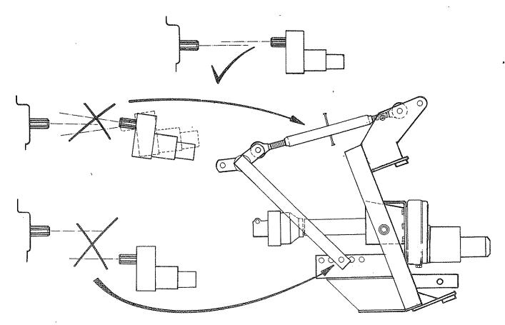
Ideally the tractor stub shaft and the gearbox shaft should be in a straight line. The greater the misalignment, the shorter will be the expected working life of the powershaft points. Parallel adjustment is affected by the top link and vertical alignment is adjusted by the hole selection between the yoke and the mainframe.
