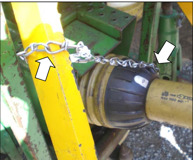
Attach torque chains to convenient locations to prevent rotation of PTO shaft guarding.
