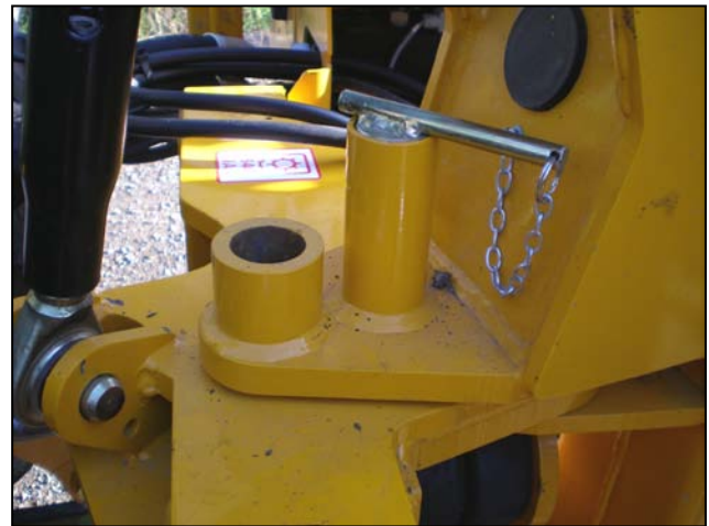
Slew Unlocked – only for working
