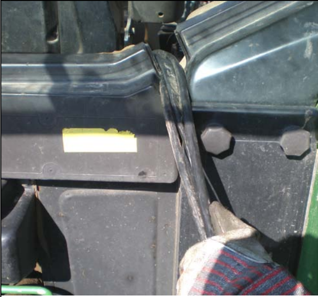
Feed control lines into tractor cab – avoid sharp bends and keep lines well clear of all moving parts on the machine or tractor.
