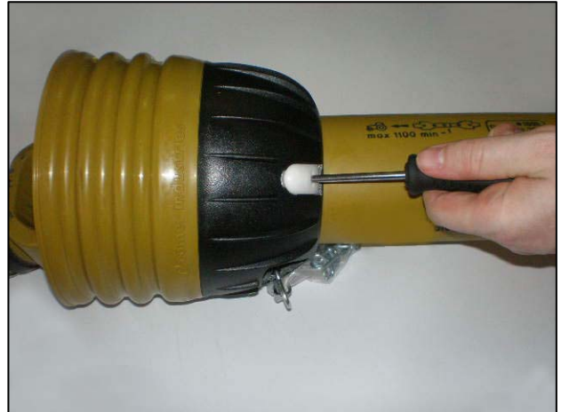
Insert screwdrivers into the clasps
