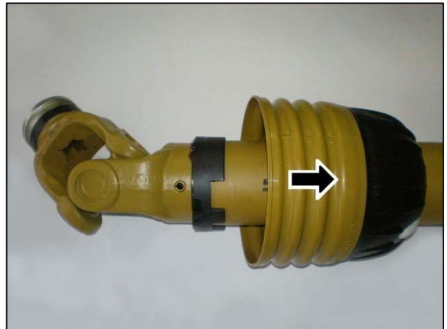
Slide shield back to reveal universal joint
