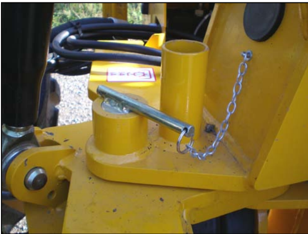
Slew Locked – always for transport & storage
