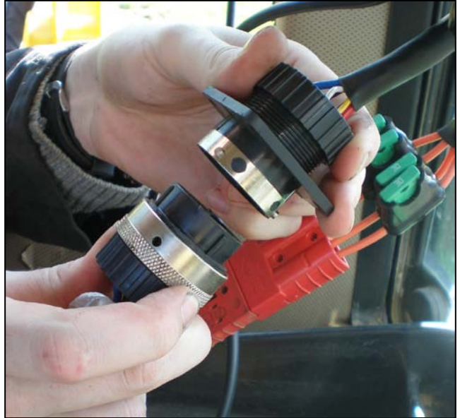
Connect control lines to the machines control unit in the tractor cab.
