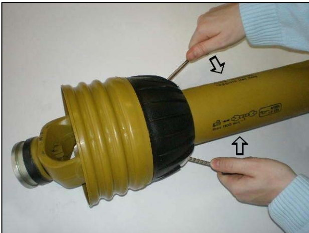
Prise clasps open to release the shield
