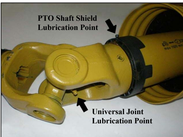
Location of lubrication points
