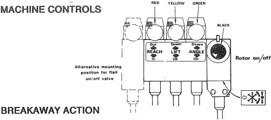
When the flail head meets an obstruction and the tractor continues to move forward, the complete armhead which is hinged on the frame will be forced backwards and upwards at the same time in an effort to clear the obstruction. Resetting of the breakaway is completely automatic with the armhead returning to its working position under its own weight. Breakaway reset forces are absorbed by rubber damper.
