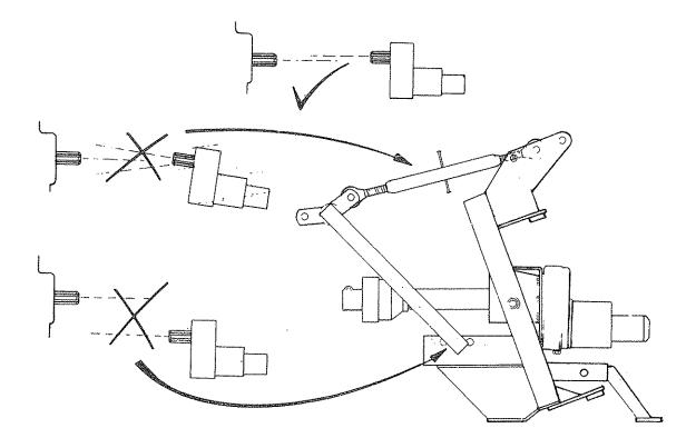
Remove the parking feet, turn inward 90 degrees and re-locate in their housings.
