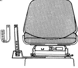
Illustration shows control unit arrangement for fully independent models with extra control handle for rotor ON-OFF. This handle can be mounted either end of the main control block to suit individual operator requirements.
