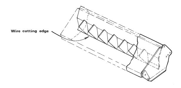
Both flail hoods are equipped with a wire trap. The trap consists of a steel plate welded across the underside. Any loose ends of wire which are picked up and carried round by the rotor are cut by the edge of the metal plate and fall harmlessly to the ground. This plate should not be interfered with or modified in any way.
