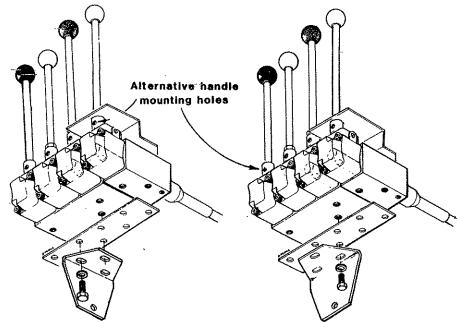
The control unit itself is bolted to an angled mounting bracket in either a transverse or longitudinal position thus giving a variety of mounting positions, which in conjunction with the flexibility of the mounting pillar will enable a satisfactory working position to be achieved.
