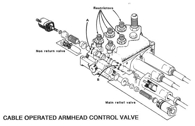
Replacing damaged or worn spool 'O' rings.
