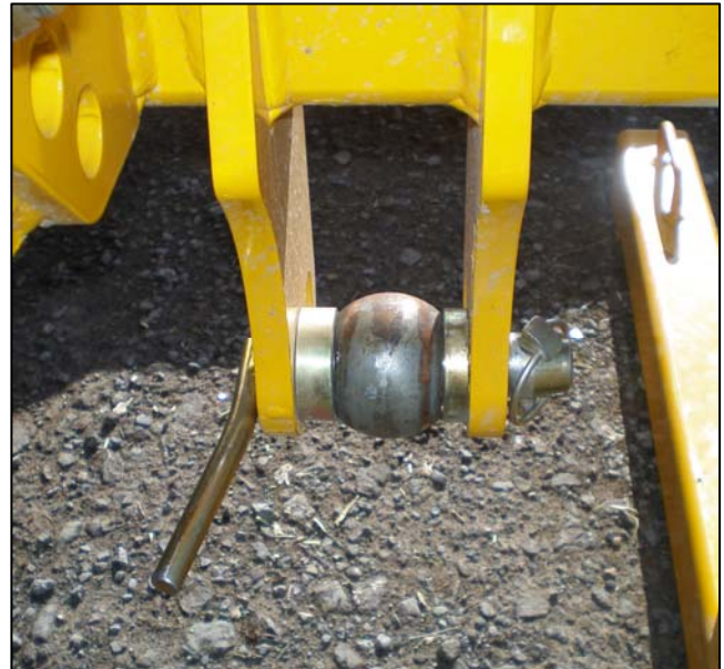
Fit lower link balls and spacers into lower frame connection points and secure with linkage and lock pins – place spacers to position lower link balls for best alignment with tractor lower links.
