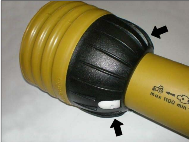
Shaft shield fixing clasps
