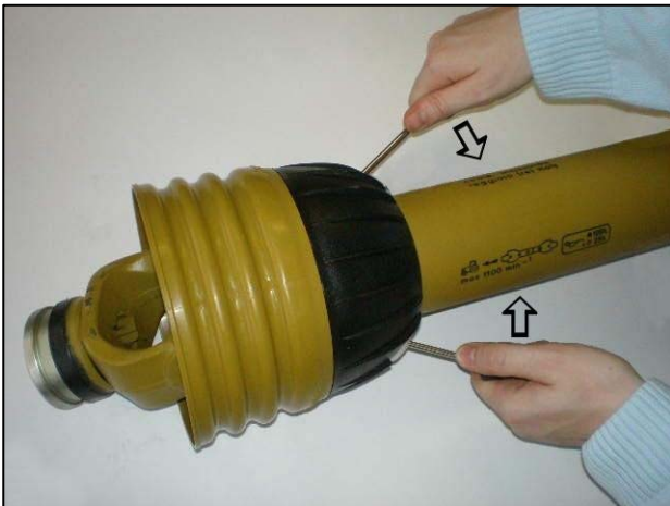
Pry clasps open to release the shield
