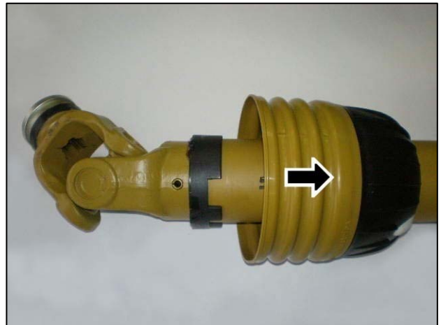
Slide shield back to reveal universal joint
