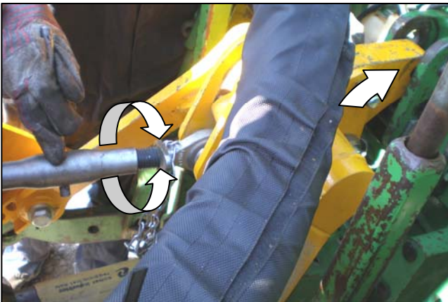
Adjust top link to position the stabiliser tongue for attachment to the tractors top link clevis. NOTE: Alternative tongues for stabilisers are available for differing applications.
