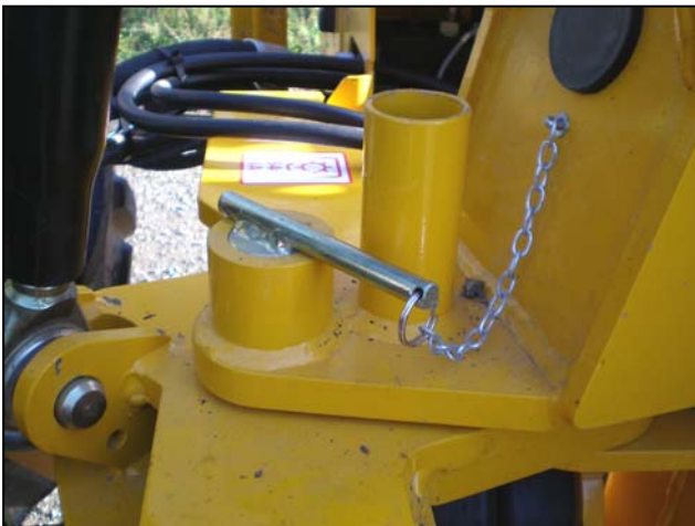
Slew Locked – always for transport & storage
