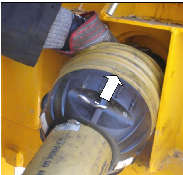
Fit PTO shaft to the stub axle of the machines gearbox – NOTE; for initial installation of a new machine or attachment to a different tractor refer to PTO note at top of page.
