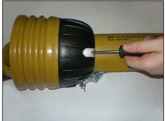
Insert screwdrivers into the clasps
