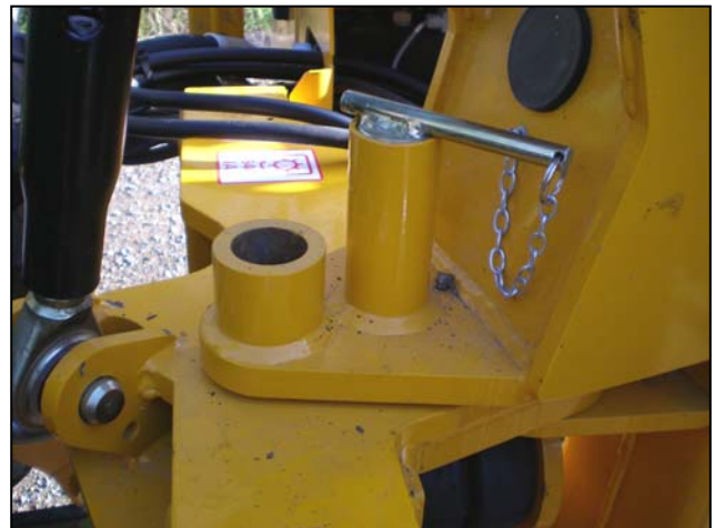
Slew Unlocked – only for working
