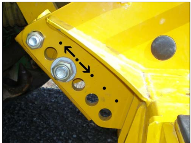
IMPORTANT: Rear of stabiliser tongue should be as close as possible to the bottom of the stabiliser slot with the machine at rest on the ground – if required change the stabiliser lower attachment points and/or clevis attachment position to achieve this setting. This is a vital requirement to ensure the tongue is located at the slots mid-point when the machine is raised to the work position thus allowing float in each direction.
