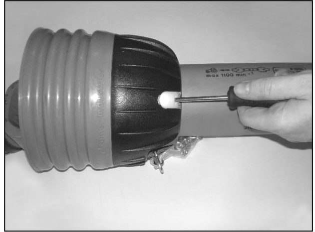
Insert screwdrivers into the clasps
