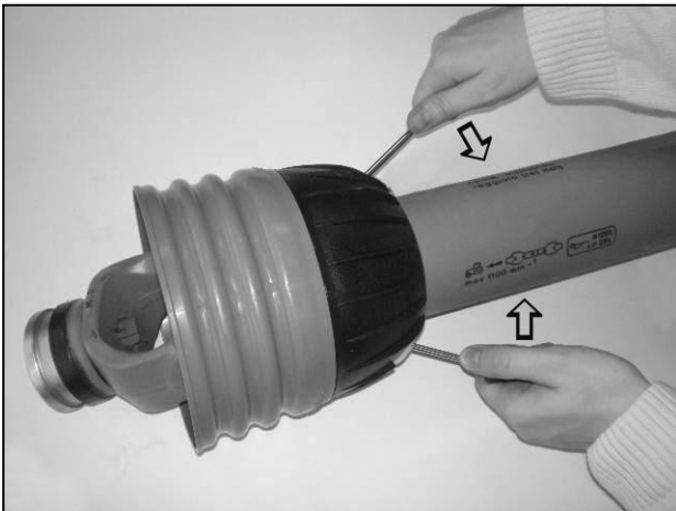
Prise clasps open to release the shield
