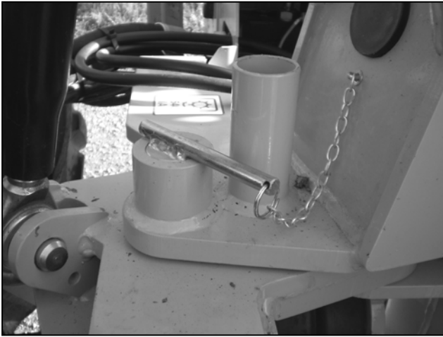
Slew Locked – always for transport & storage
