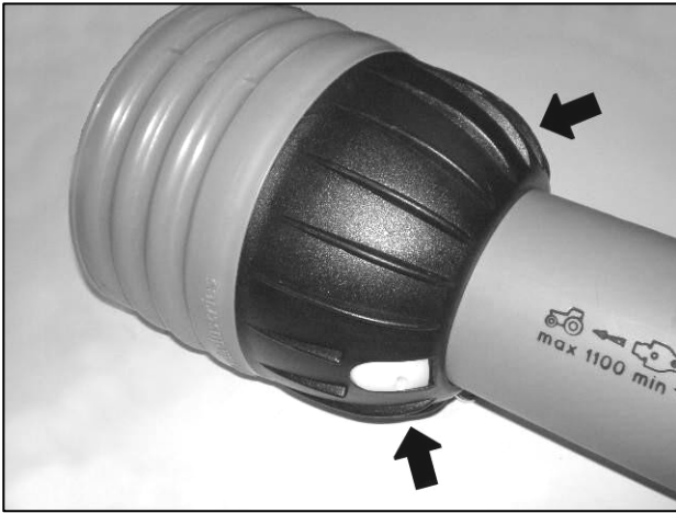
Shaft shield fixing clasps
