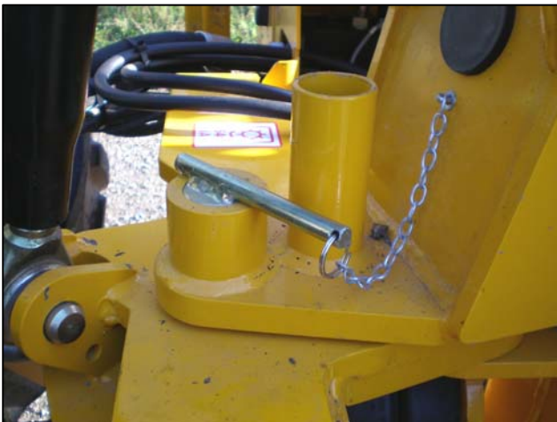
Slew Locked – always for transport & storage
