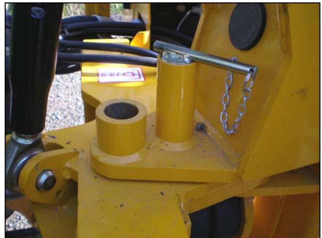
Slew Unlocked – only for working
