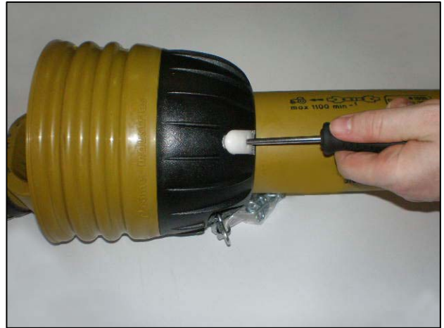
Insert screwdrivers into the clasps
