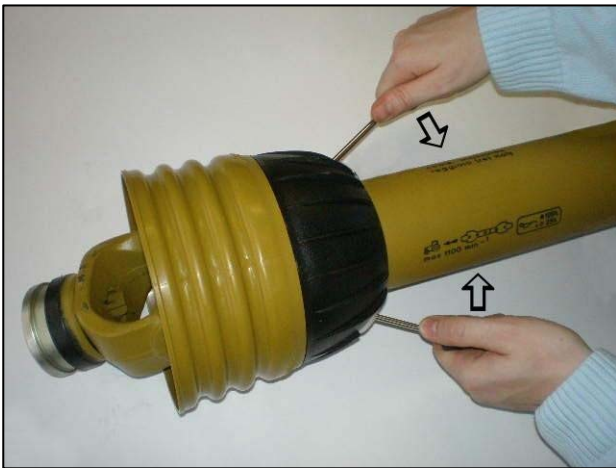
Prise clasps open to release the shield
