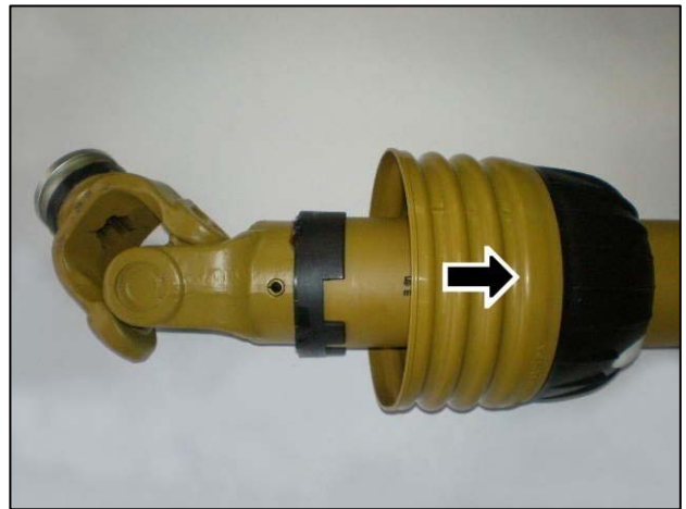
Slide shield back to reveal universal joint
