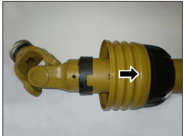
Slide shield back to reveal universal joint
