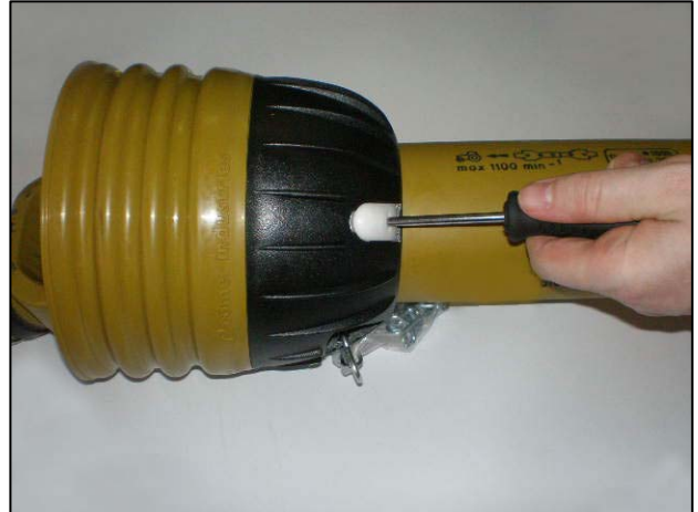
Insert screwdrivers into the clasps
