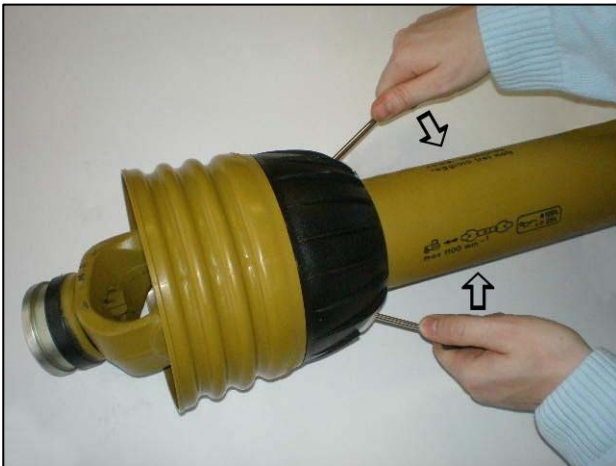
Pry clasps open to release the shield
