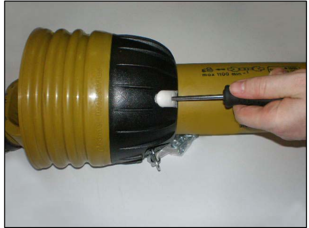
Insert screwdrivers into the clasps
