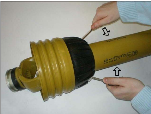
Prise clasps open to release the shield
