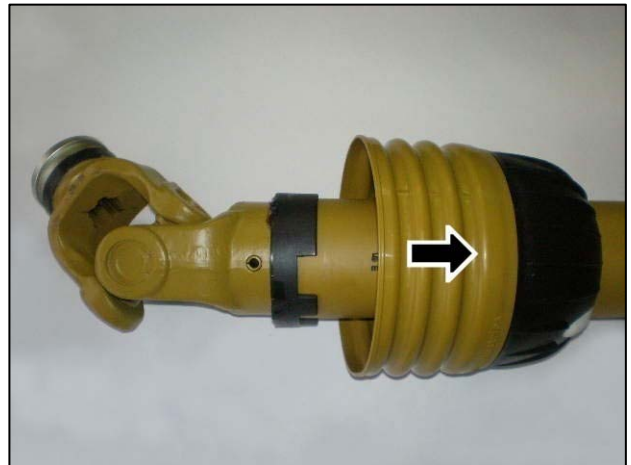
Slide shield back to reveal universal joint
