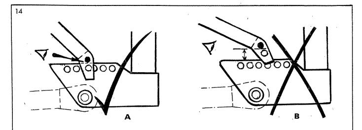
B Check the welded in pins between the stabiliser jaws are in contact with the mounting rail. If not the machine must be lowered to the ground and the next higher hole on the stabiliser quadrant selected, the machine raised and contact checked. Repeat again in the third hole if necessary. On subsequent fitting to the same tractor the hole selected is always used.
