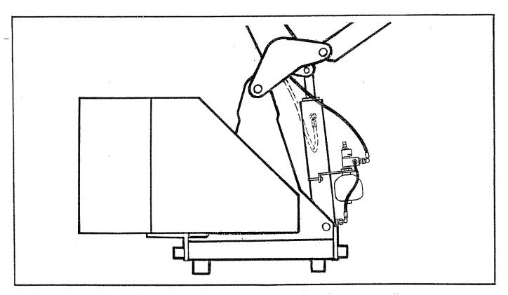
The hydraulic float kit should be mounted as shown clamped to the lift ram barrel in such a position that it does not foul any other component during work
