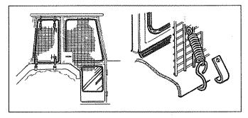
can demonstrate that the penetration resistance is equivalent to, or higher than, that provided by mesh/polycarbonate glazing. If the tractor has a roll bar only, a frame must be made to carry both mesh and polycarbonate glazing.
