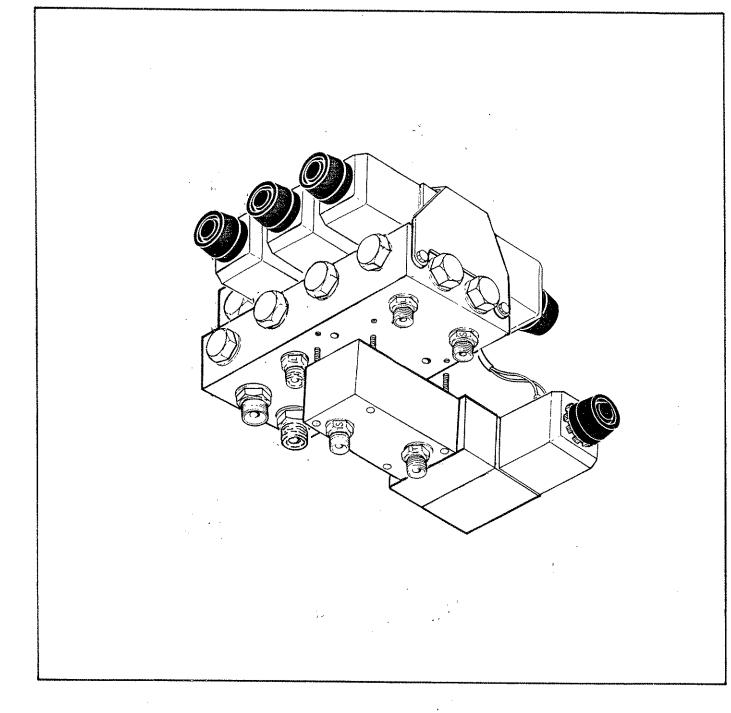
HEAD ANGLE FLOAT KIT - Optional extra on all electric controlled models.
