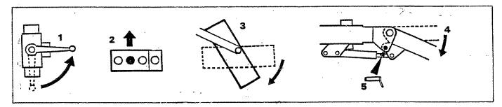
Raise the lever on the park selector diverter valve to the 'up' position.
