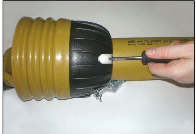
Insert screwdrivers into the clasps
