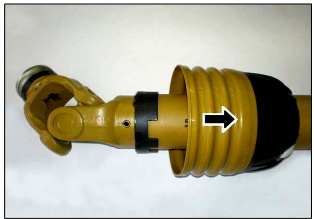
Slide shield back to reveal universal joint
