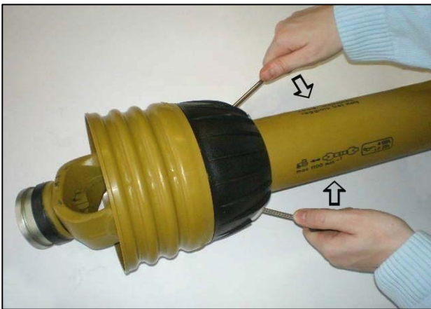
Prise clasps open to release the shield
