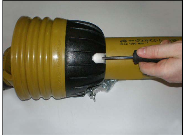
Insert screwdrivers into the clasps
