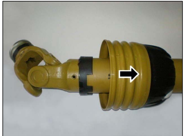
Slide shield back to reveal universal joint
