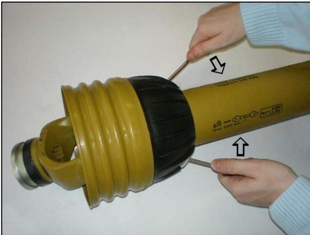
Pry clasps open to release the shield
