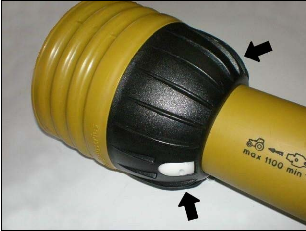
Shaft shield fixing clasps
