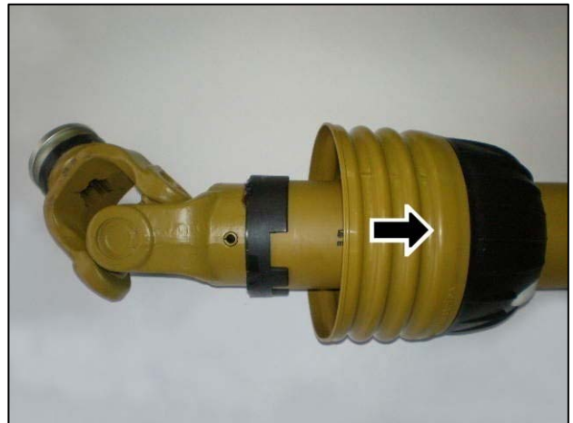
Slide shield back to reveal universal joint
