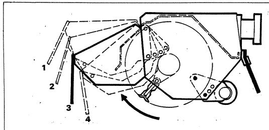
A front hood c/w flaps and a rear flap must be fitted. The front hood must to set in the lowest position which allows the material to be cut. The roller may be set in positions 2 or 3.
