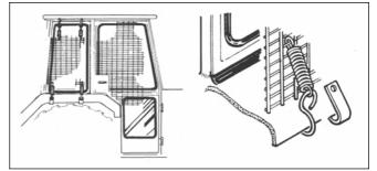
can demonstrate that the penetration resistance is equivalent to, or higher than, that provided by mesh/polycarbonate glazing. If the tractor has a roll bar only, a frame must be made to carry both mesh and polycarbonate glazing.
