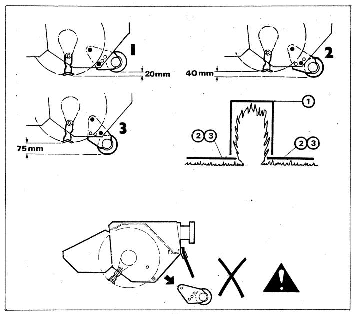
LIFT FLOAT KIT (Optional extra for ground cutting on flail machines only).
