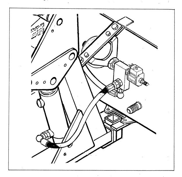
The hydraulic float kit, if fitted, should be mounted as shown bolted to the tank stay strap.
