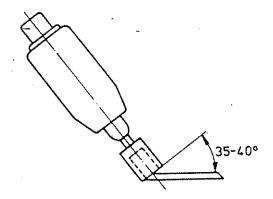
A cutting angle of 35 degrees - 40 degrees is required.
