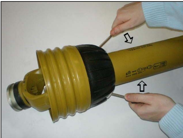
Prise clasps open to release the shield
