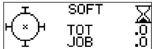
5. Pressing ✓ while the EDS is turned on will scroll through the **SOFT**, **MED** and **HARD** working settings.
