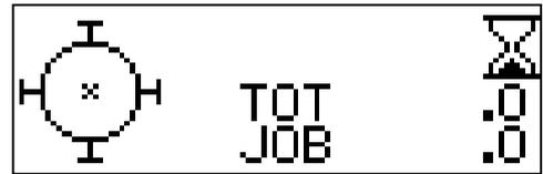
3. Pressing either of the Rotor ON buttons will activate the 'egg timer' and rotor image.
