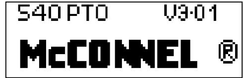
2. Pressing scroll forward once will display the running screen. The **TOT** displays the total time the rotor has been switched on. The **JOB** also displays the rotor on time but may be reset to zero by pressing the **X** button for 3 seconds.
